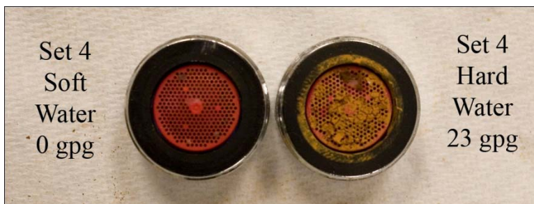
Figure 5-22. Photo showing the Set 4 faucet strainers at the end of the test.
